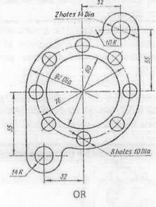
Q.1(B) Draw the figure shown below using Auto CAD commands and dimension it.
