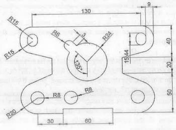
Q.1(B) Draw the figure shown below using Auto CAD commands and dimension it.
