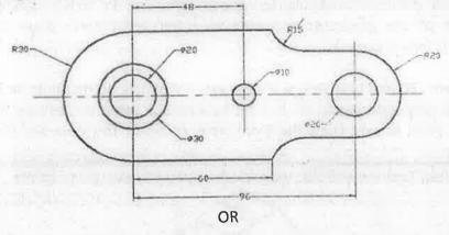
Q.1(B) Draw the figure shown below using Auto CAD commands and dimension it.
